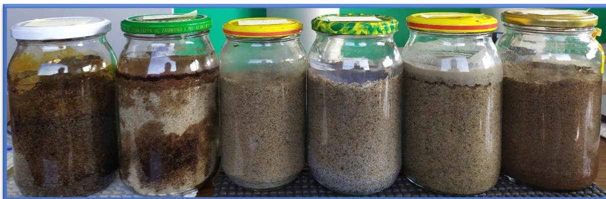
Fig. 2. Visual effect of waste-based stabilisers affecting the soil sealing influencing its frost resistance
